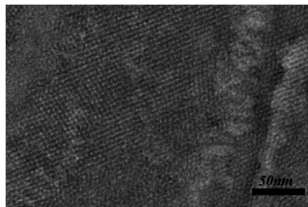
Figure 2. TEM image of well-ordered mesoporous cubic aminosilica after ammonolysis at 550 °C for 4 h.
